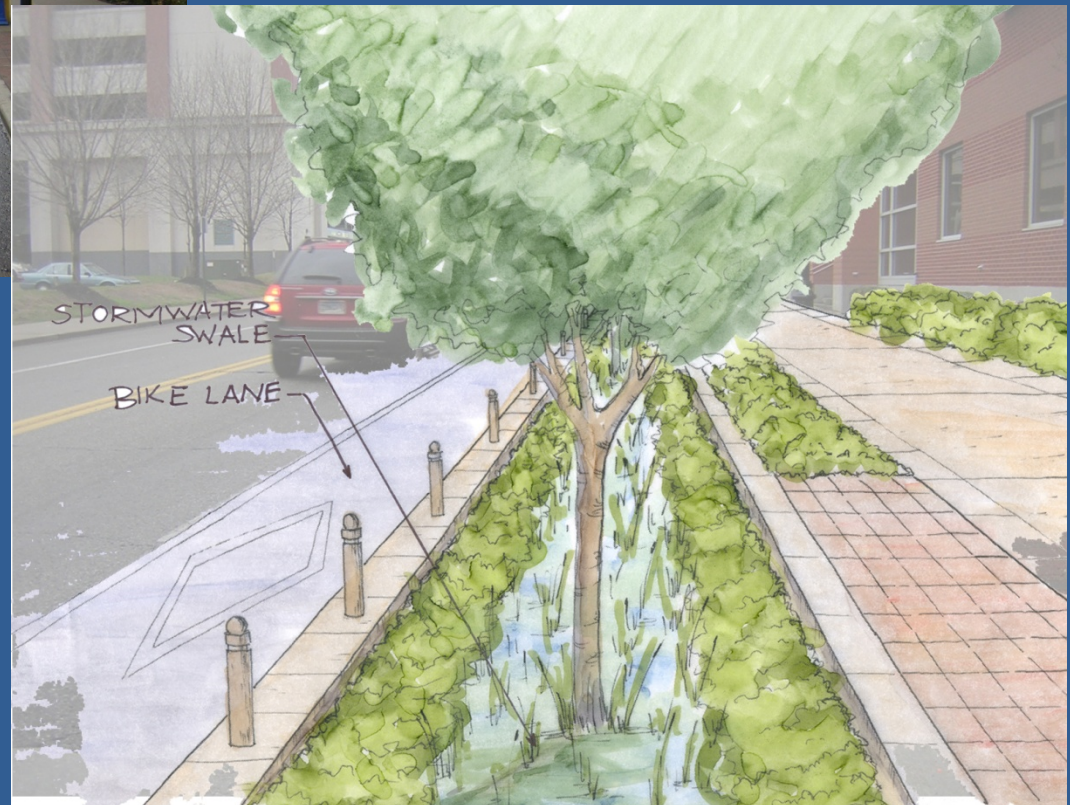
AFTER: Madison Avenue with Stormwater Swale
